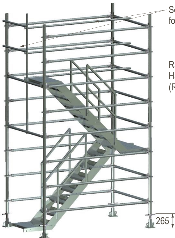
Stair Units fitted within a 1500x2400mm Rapidshor tower (Bracing omitted for clarity)
