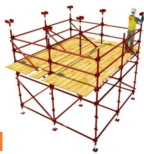
Working from the boarded platform adjust the Adjustable forkheads to approximate required jack extension and insert into the top level of open ended standards.
