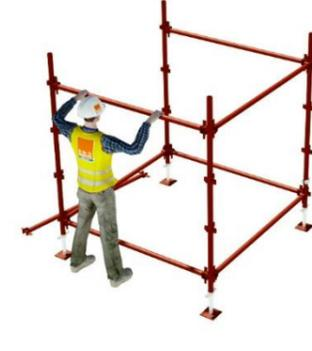
The first unit of the grid is completed by tying the legs to one another with ledgers to the required set of pressings on the standards and levelling-off and squaring up. Once this is completed, wedges are hammered up tight. Always refer to RMD Kwikform design drawings.
