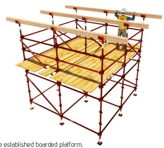
Working from the established boarded platform, insert primary beams into the centre of the forkhead. Twist the forkhead and insert wedges to ensure the primary beams are central.
