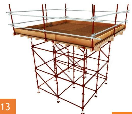
Place the plywood and secure to secondary beams using suitable screws or nails. Erect perimeter guardrails and toe boards to comply with local safety regulations.
