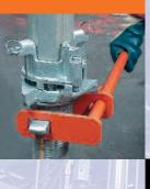
The unique load release mechanism gives a quick and effective release of load, allowing easy rotation of jack collar, without the need for spanners. This also eliminates the regular maintenance and damage problems experienced with systems without this feature.
