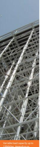
Variable load capacity up to 120kN/leg, depending on number of frames in height, extended length of screw jack and overall height of propping, allows economic designs through many assembly options, by choosing different grid sizes and the minimum number of ledger frames in height.
