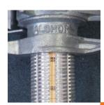
Integral measuring tape embedded in the screw jack ensures accuracy of build, speeding-up assembly and inuse adjustment.
