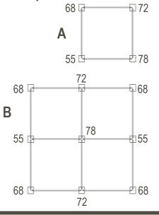
Individual Tower A is shown with the calculated leg loads in the tower. The maximum leg load is 78kN. Use a design leg load for this tower of 78kN.
