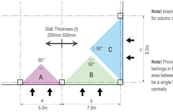
**Note!** bracing/lashing not required for column centres of <6.0m
