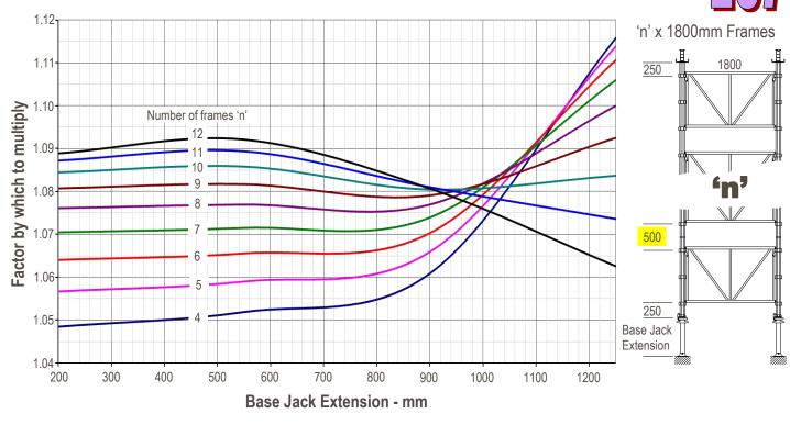
Note: Ensure that the base jack bears on a foundation that is restrained against rotation, e.g. a concrete slab or railway sleepers haunched with concrete
