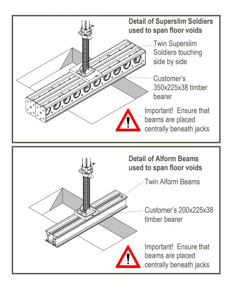
Maximum allowable leg load for both configurations is 80kN.
