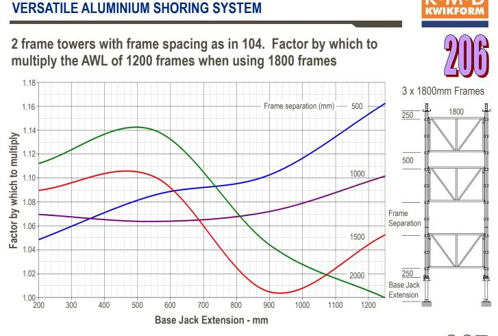
Factor by which to multiply the AWL of 1200 frames when using 1800 frames for 500 separation between frames
