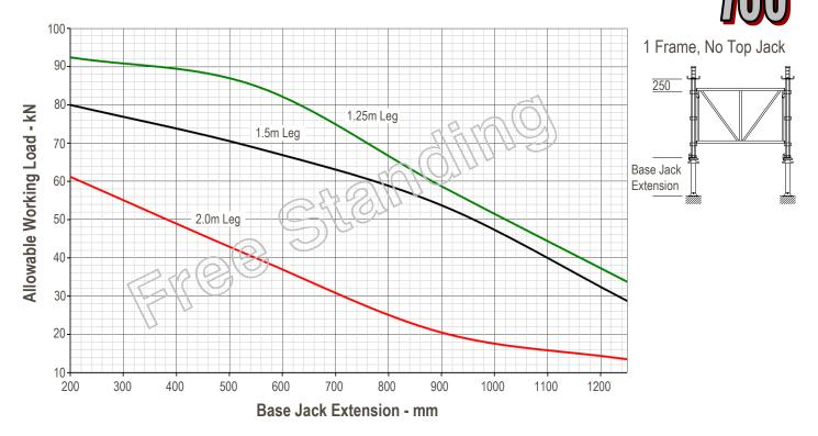
Free-Standing Alshor Plus Towers with 2.5% Side Load Applied at the Top. Base Fixed in Rotation & Head Pinned with a Load Eccentricity of 5mm (fos = 2.0)
