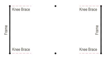
Plan Showing Leg, Knee Brace & Frame Configuration
