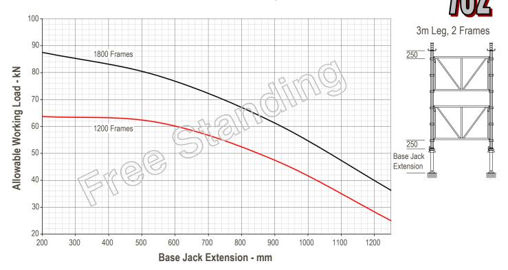
Note: Ensure that the base jack bears on a foundation that is restrained against rotation, e.g. a concrete slab or railway sleepers haunched with concrete
