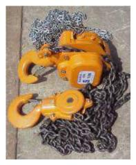
Adjustable Chain Block (5 tonnes pull lift)
