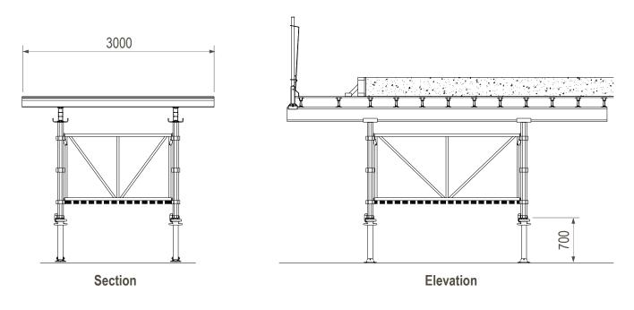
The Alshor Plus consists a 1500 leg with no top jack & a Base Jack extended 700mm. Whilst a detailed assessment of the individual leg loads is warranted, for this example a basic analysis is shown below;-
