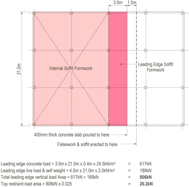
Concrete pressure load =  $50\% \times 21.0m \times (23.5kN/m^3 \times 0.4m/2 \times 0.4m) =$ 19.7kNDesign top restraint load for leading edge soffit formwork=20.2kN + 19.7kNTotal load in bracing/ratchet lashings at  $45^\circ = 39.9kN \times \sqrt{2}$ =56.4kN
