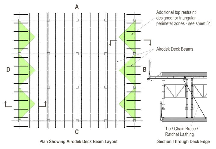
Building edges A & C have continuous runs of Deck Beams transferring edge top restraint loads into the internal soffit area. Design ties/braces/ratchet lashings only to prevent edge Deck Beams from tipping over.
