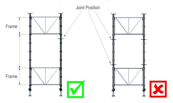
Provided there is one level of frames attached to each level of legs then intermediate frames are permitted to span over the joint in the leg.
