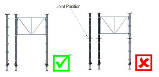
Structures designed with multiple frames in the height shall have no more leg sections in height than the number of frames. At least one level of frames fully attached to each lift of legs etc.
