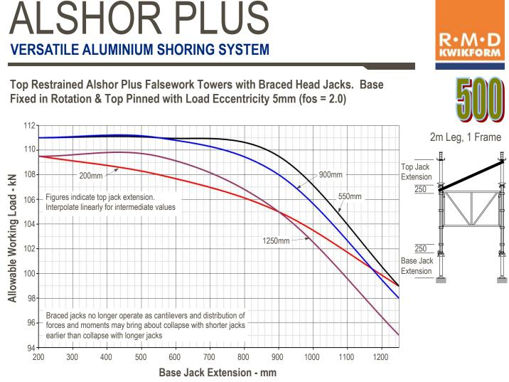
**Note:** to avoid clashing jacks when using the 2m Leg, the minimum combined jack extensions must be greater than 1375mm when using 2 No. long jacks and 625mm using a long jack at the base with short jack at the head.
