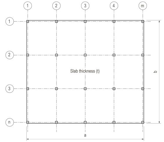
Vertical load due to concrete: **abtp**. Where  $\rho$  is the density of the concrete, usually taken as 24.5 kN/m<sup>3</sup>. Vertical load due to live load and self weight of equipment = 2.0kN/m<sup>2</sup>.
