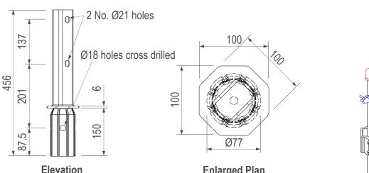
**Enlarged Plan** Alshor Plus Node Lug (ASX10052) weight 1.65kg
